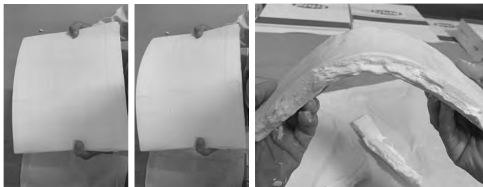
Slika 6. Ispitivanje elastičnosti margarina kristalizovanog kroz tri rashladna cilindra Figure 6. Elasticity test of margarine crystallized with three cooling cylinde
