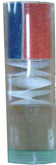
Figure 3. Rotation of the revolving static mixer.
