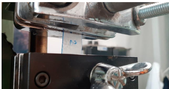
Figure 3. Measurement of the angle of torsion.
