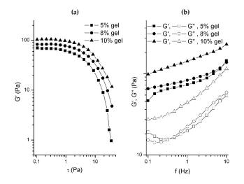
**Figure 1.** Rheological properties of chia seed hydrogels of different concentrations presented with (a) stress sweep and (b) frequency sweep curves.
